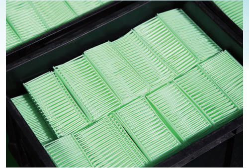
In-House Injection Molding Process for Swab Handle ( Inspected Molded Handle )
