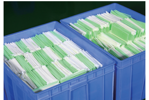
Finished Swab Head Process ( Sent for Final Inspection on Swab Head and Handle )
