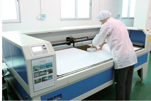
Laser Cutting Process ( For Polyester and Microfiber Fabric )
